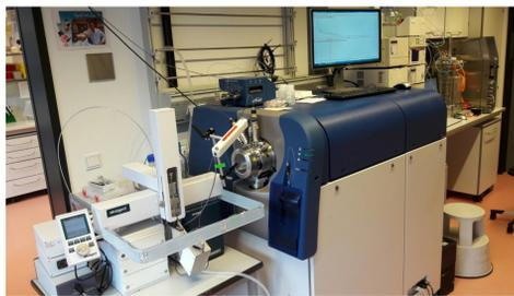
Figure 1: LC-MS-System (TripleToF 4600) used for MRM-Investigations of PCCs and coagulation factors
